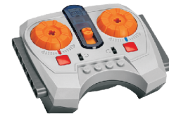
8879 IR Transmitter with inversion and 7-steps speed control
